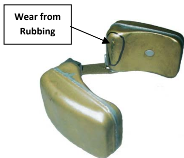
Example: Wear from Rubbing on Small MA Float
