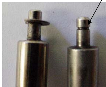
Figure 5 Close up detailing lack of wear on good stems.
