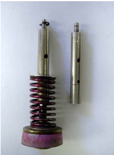
Figure 4 Two good accelerator pump stems, one with clip still installed.
