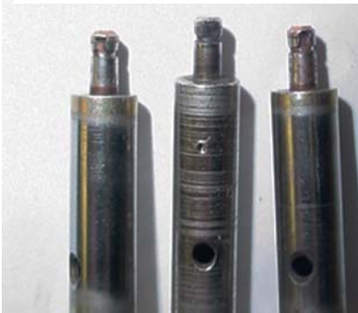
Figure 1 Three bad Accelerator Pump Stems.
