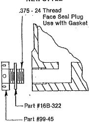
Pipe Plug style drain plugs and face seal style are not interchangeable. It is easier to remove and install the #99-8 Hex Head type when you service the old style.
