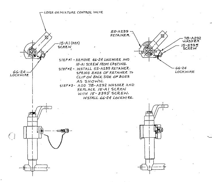
Lightly coat the tip of retaining screw 15-B395 with a silicone grease at assembly.
